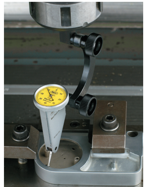
Centering of a bore
